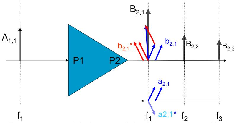
The total response of the b2 scattered signal, due to a2 is a combination of b2 and b2\*:  $b2=S22 \times a2 + T22 \times a2*$
