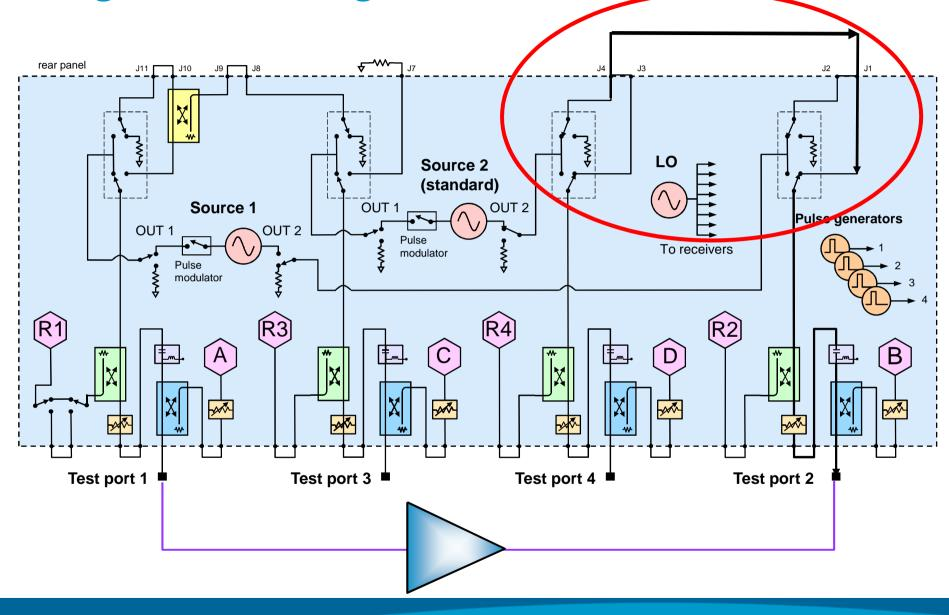
Start by driving a signal into the amplifier
