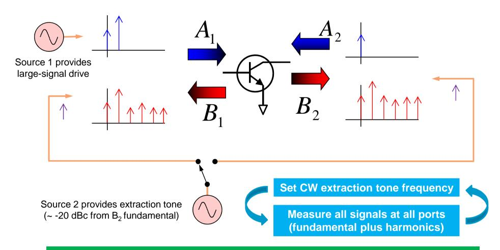
Repeat extraction-tone loop for each large-signal drive level, frequency, bias, etc.
