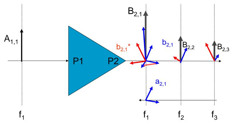
Changing the phase of a2 changes the total magnitude of b2 wave, but not the magnitude of individual parts, b2 and b2\*
